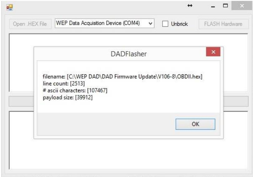
6. Press and hold the red power button on the side of the DAD unit to ensure the DAD is powered on. Release the button and click on the “**FLASH Hardware**” button to begin the update.
