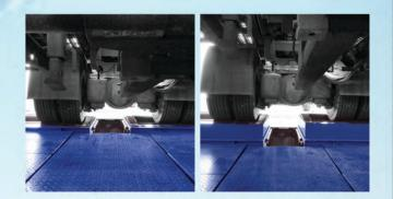
This method allows the system to apply the brake test method of extrapolation, with the scale option and optional tire pressure sensors of the vehicle braking circuit. Lift racks include two guided structures, one for each brake tester frame, which allows lifting of the rollers. Lifting is accomplished by hydraulic cylinders, and an oil hydraulic circuit made with flow dividers permits the racks to rise synchronously.
