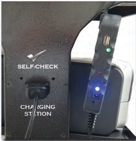
Integrated OBDII DAD Verification and Charging Station to ensure your OBDII DAD is communicating, charging, and operating properly
